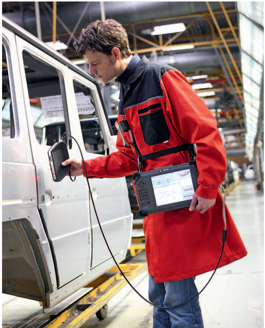
Picture 1. The angle of the measuring device to the surface is recognised and the measurement results corrected accordingly. No precise orientation of the hand sensor is necessary for the measurement.
