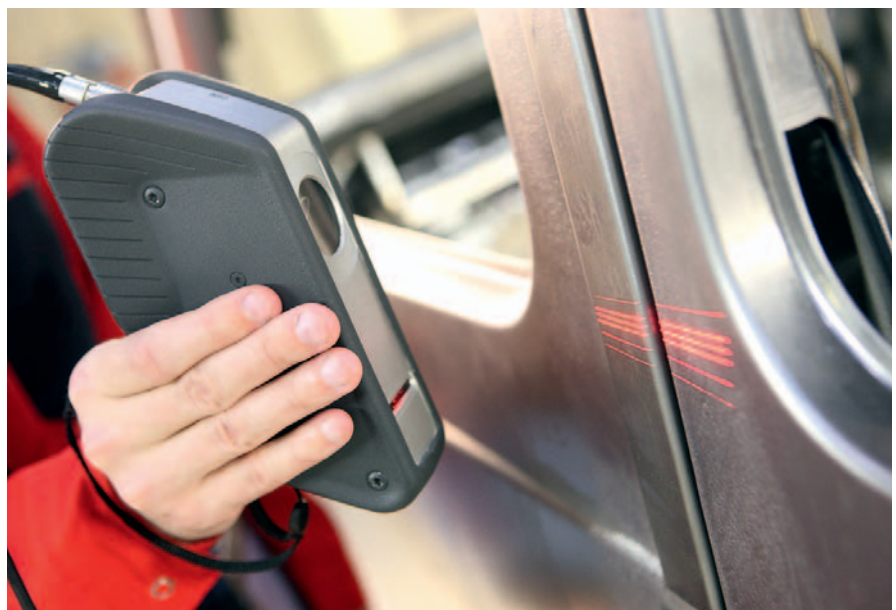
Picture 2. The gap measurements are taken throughout the entire production process, from the structural phase to painting and assembly.
